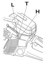
The T-screw regulates the throttle setting at idle speed. If the T-screw is turned clockwise this gives a higher idle speed; turning it anti-clockwise gives a lower idle speed.
